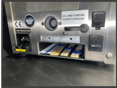
Figure 2. Photo of biological and chemical indicators placed within battery compartment of the particle counter.
