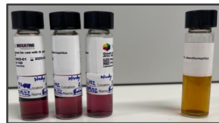
Figure 5. Biological indicators negative for growth post HHP treatment with one positive control.
