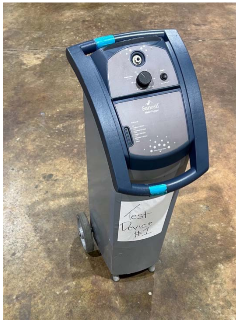
Image 3. The H 2 O 2 delivery device used for testing. This device is paired for use with the hydrogen peroxide and silver (5% H 2 O 2 / 0.01% Ag) disinfectant solution. 7
